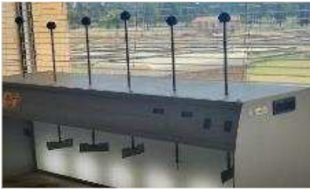
Jar Tests conducted regularly at Balkfontein WTW
